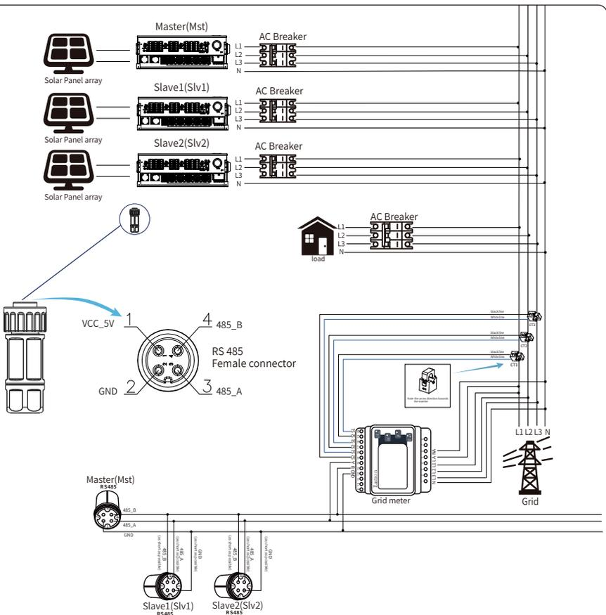
Pic 7.25 Connection diagram(Three-phase electricity )
