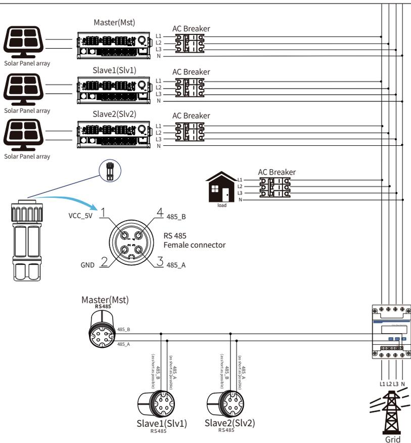
Pic 7.29 CHNT Connection diagram(The pass-through table)
