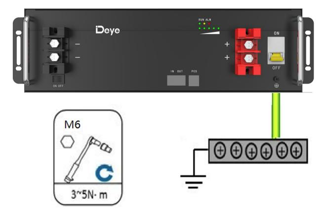
Figure 5-1: Install the Grounding Wire
