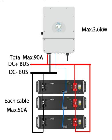
If the inverter power exceeds 3.6kW, the parallel mode must be used mode 2!
