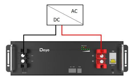
Figure 5-2: Single Battery Connection
