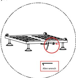
Connect one end of the ground cable to the cluster rack and the other end to the ground bar at the installation site.
