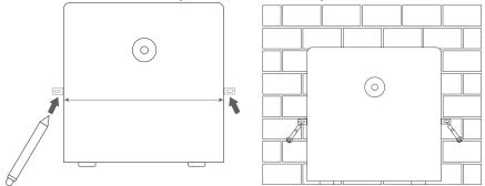
3) Adjust the left and right screws to the appropriate position to ensure that the battery is perpendicular to the ground.
