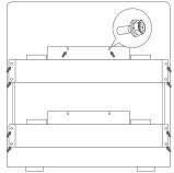
5)Carry the battery and hook it onto the hanging plate. Ensure that the upper and lower hooks of the backplane are accurately buckled on the hanging plate.
