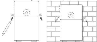
3) Adjust the left and right screws to the appropriate position to ensure that the battery is perpendicular to the ground.
