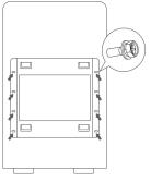
5)Carry the battery and hook it onto the hanging plate. Ensure that the upper and lower hooks of the backplane are accurately buckled on the hanging plate.
