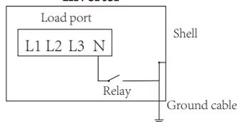
**Asymmetric phase feeding:** If it was checked, the inverter will take power from the grid balance of on each phase (L1/L2/L3) when needed.
