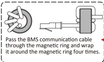
Pass the BMS communication cable through the magnetic ring and wrap it around the magnetic ring four times.
